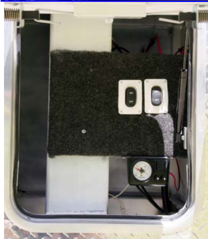
Above is the air-ride leveling control. Simply pump up the low side and bleed air from the high side. We have an 12v electric 120 psi pump and reserve air tank.
